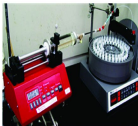
DECON Column-Sorption Column:Bi-16 \mu\text{L}/\text{min} , 100 \mu\text{M} MPT, 70 h
