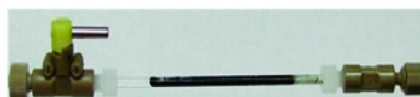
100 mg MOF powder packed in column 2.5 mm I.D., length: 125 mm in Length
